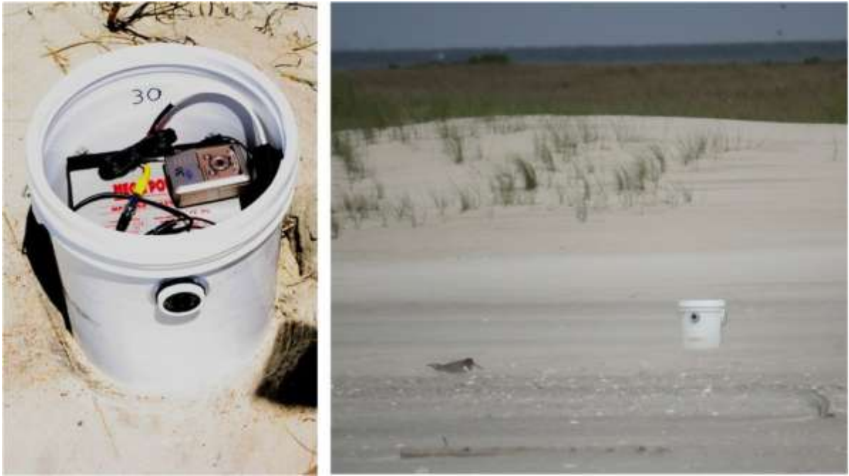
Figure 2.1. Video recording equipment used to monitor incubating American Oystercatchers and surrounding beach activity. The recording system consisted of a camera, digital video recorder, and batteries encased in a white 5-gallon plastic bucket (left). A camera unit deployed at an active oystercatcher nest at North Core Banks, Cape Lookout National Seashore, NC (right).
