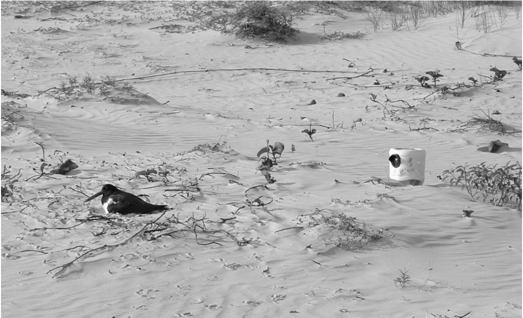
Fig. 2. Each camera was mounted on a wooden stake, placed approximately 1.5–2 m from a nest, and protected by a cutout plastic bottle. An 18.3-m cable buried 2–3 cm in the sand substrate connected each camera to a recorder and battery.
